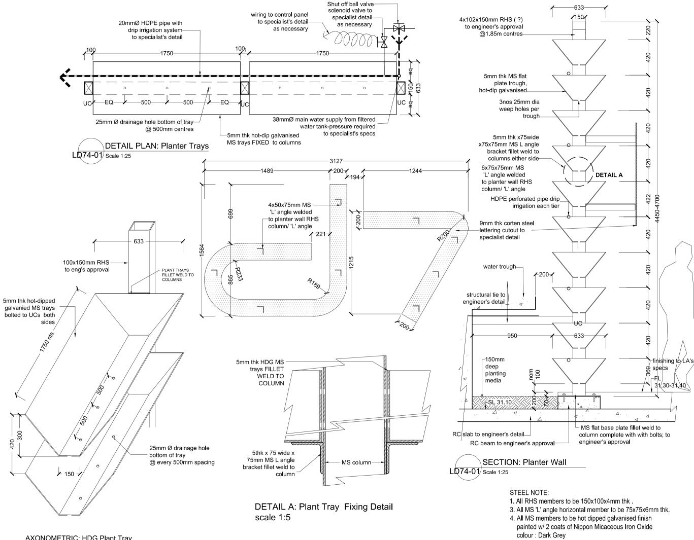
AXONOMETRIC: HDG Plant Tray scale 1:10
